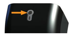
2. When the S200 has booted up, press the Wi-Fi input button on the side of the S200 (item 5 on page 3).
